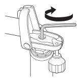
**4** Using a 5mm hexagonal key wrench to tighten the stem bolt. The stem bolt is properly tightened when the handlebars cannot be twisted out of alignment with the front wheel. Make sure the handelbars are in line with the front wheel before tighten stem bolt all the way.
