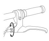
**1** To adjust the brake cable wire, thread the brake lever adjuster in or out 1/4 to 1/2 turn until the desired cable tension is attained
