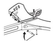
**3** Insert the two coupling bolts and two hexagonal bolts. Starting underneath with the bolt on the back. Turn product over and insert the next set of bolts. Tighten with two 5mm hexagonal wrenches.
