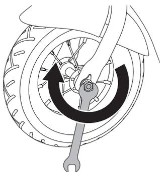
**4** Tighten the nuts using two (2) 14 mm wrenches.
