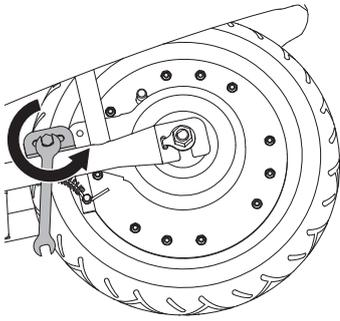
**4** Using two (2) 8 mm wrenches, loosen and remove the bolt and lock nut from the cable guide bracket.
