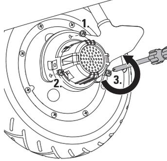
**2** Using a Phillips screwdriver, loosen and remove three (3) screws from motor cover.
