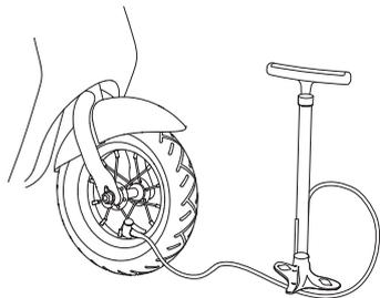
Using a bicycle tire pump equipped for a Schrader valve, inflate the tires to the PSI indicated on the sidewall of the tires.
