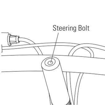
**1** Using a 6 mm Allen wrench, loosen steering bolt in four (4) complete turns so that the wedge is loose and not touching steering tube.
