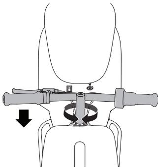
**3a** While inserting the steering tube down into the handlebar tube, hold steering bolt steady with thumb and rotate handlebars 180 degrees in either direction making sure not to pinch any cables.
