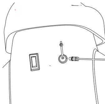
**2** Make sure the power switch is in the **OFF** position. Plug the charger into the charger port on the product. The light on the charger should turn red during charging. The light will turn green when charging is complete.
