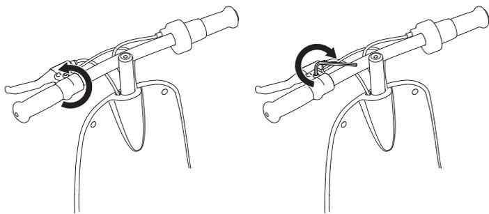
**1** Adjust angle of the brake lever to a comfortable position for the rider by turning back and forth.
