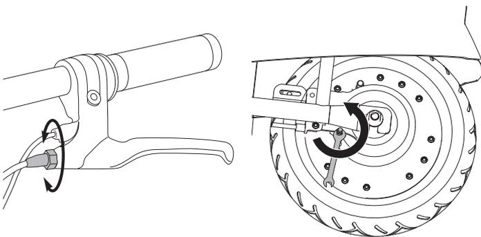
**1** To adjust the tension, thread the brake lever adjuster on the hand brake in or out 1/4 to 1/2 turn until the desired brake adjustment is attained. Most adjustments are complete at this step. If brake still needs further adjustment, proceed to step 2.
