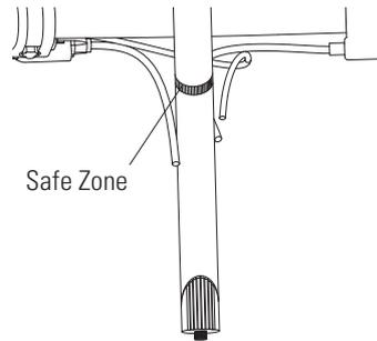
**4** Slowly slide the handlebars up to make certain that the bar is in the "SAFE ZONE". Failure to secure the handlebars within the "SAFE ZONE" can cause the handlebars to come out while riding.
