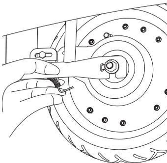
**7** Thread the brake cable through the brake adjuster barrel, through the large spring, and into the small hole in the side of the anchor bolt. Position the cable to the original location (as indicated by the slight cable kink) and tighten securely.
