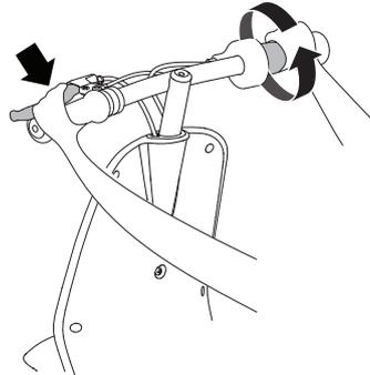
**Note:** As an additional safety feature, the Pocket Mod Petite is designed to cut power to the motor when the hand brake is applied.
