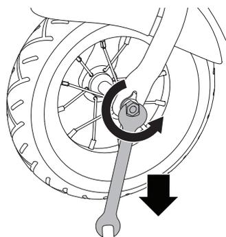
**1** Remove the nuts on both sides of the front axle using a 14 mm wrench then remove the lock washers and remove the wheel from the fork.
