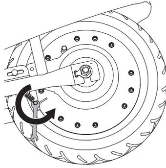
**3** With a 10 mm wrench, loosen the brake cable anchor and disconnect the cable.
