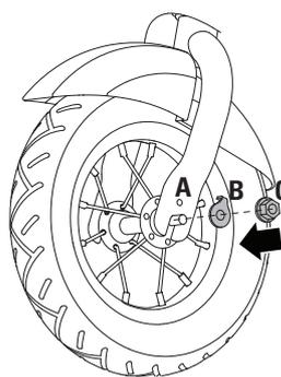
**3** Insert tab on the lock washer (**B**) into the hole (**A**) on the front fork and then place the nuts (**C**) on top of the lock washer (**B**).
