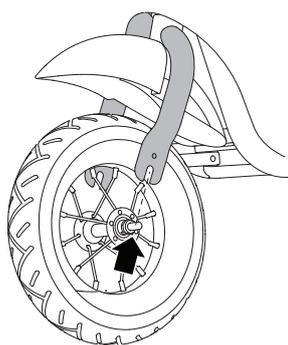
**2** Insert the new wheel into the front fork with the lock washers on the outside of the fork. See step #3.
