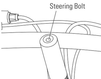
**5** Securely tighten bolt using 6 mm Allen wrench.
