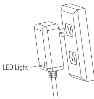
**1** Plug the charger plug into wall outlet. The light on the charger should be green.
