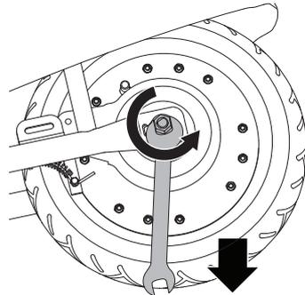
**5** With 17 mm wrench, loosen the nut. Remove wheel/hub motor.
