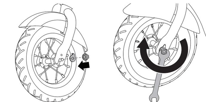
**4** Insert the tab on the lock washer into the hole on the front fork.
