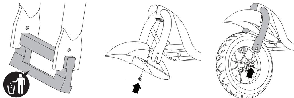
**1** Remove the plastic packing material from the front fork.
