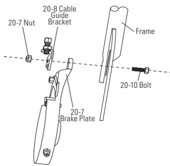
**6** Install the cable guide bracket to the frame and brake plate using bolt, washers, and nut. Do not tighten.
