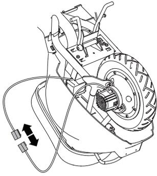
**1** Locate and disconnect motor from controller.
