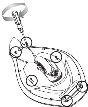
**4** Re-attach the deck plate to the platform with the six (6) Phillip screws removed in step 1.
