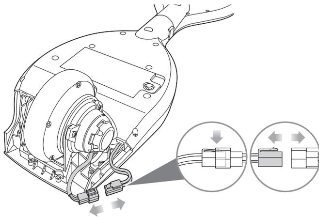
**2** Disconnect the motor connector from the control module.
