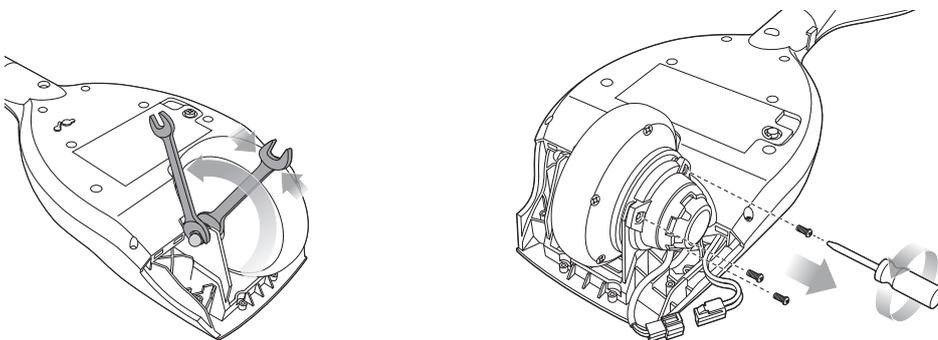
**3** Using a 13 mm wrench, loosen the outside locknut (11-6). Use a 13 mm wrench to prevent the inside nut (11-3) from turning.
