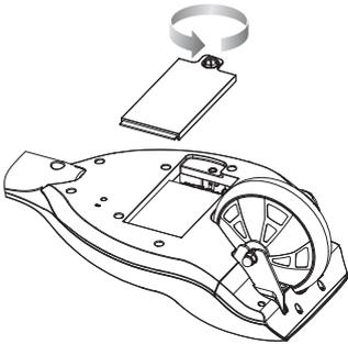
**1** Turn product over. Loosen the Phillips screw on the battery cover and remove cover.
