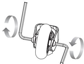
**1** Turn product over. Using two (2) 5 mm Allen wrenches, loosen coupling bolt and remove wheel from caster.
