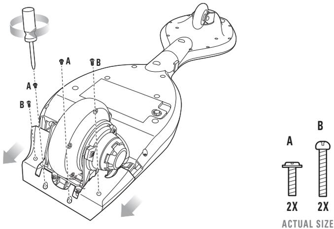
**1** Turn product over. Loosen the four (4) Phillip screws on the rear platform cover and remove cover.
