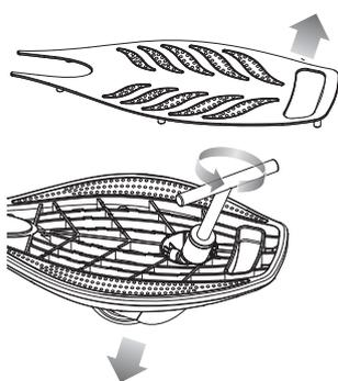
**2** Turn product over. Using a 24 mm socket wrench, loosen the nut on the caster and remove caster.
