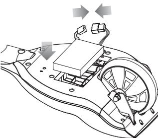
**3** Install replacement battery. Re-connect the battery connector to the control module.
