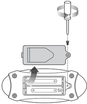
**1** Loosen Phillips screw on battery cover and remove cover. Remove old batteries and properly dispose.
