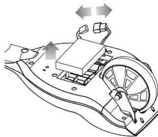
**2** Disconnect the battery connector from the control module and carefully remove the battery from product.
