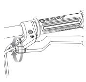
**1** To adjust the brake cable tension, thread the brake lever adjuster in or out 1/4 to 1/2 turn until the desired brake adjustment is attained. Most adjustments are complete at this step. If brake still needs further adjustment, proceed to step 2.
