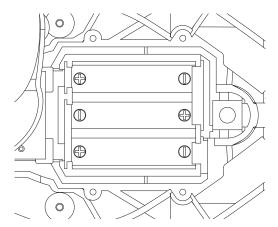
**Note:** When installing the batteries, please pay attention to the batteries' positive and negative side which must align with the positive and negative markings in the battery housing.
