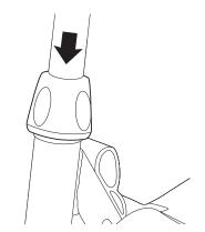
**6** Slide the steering clamp cover down and over the "E" shape fixed pin.
