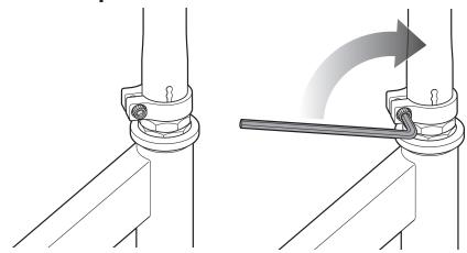
Using a 5 mm Allen wrench, check that the collar clamp bolt is tightened securely. This item is tightened and quality inspected at the factory, but there is a slight chance that the effects of shipping or handling may have caused the bolt to loosen.
