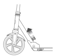
**1** To fold scooter you must first deactivate the anti-rattle feature. Twist the knob left until loose. No need to loosen knob more than one full turn.
