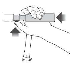
**2** Insert and secure the left and right handlebars by pressing the spring-loaded buttons and inserting them into the T-bar.
