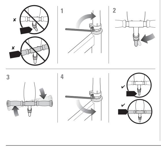
**A WARNING:** Failure to properly install and tighten the collar clamp may cause the rider to lose control and fall. If you are having difficulty understanding these instructions, please contact Razor Customer Service for assistance.
