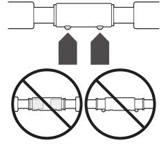
**3** Make certain **BOTH** handlebars are properly locked onto the T-bar.
