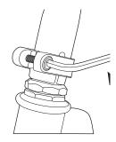
Using a 5mm Allen wrench, check that the collar clamp bolt is tightened securely. This item is tightened and quality inspected at the factory, but there is a slight chance that the effects of shipping or handling may have caused this bolt to loosen.
