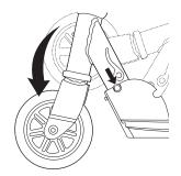
**Note:** The Joint lever is springloaded and will automatically lock in the upright position when fully upright.
