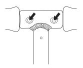
**2** Make certain **BOTH** handlebars are properly locked onto the T-bar.
