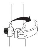
**4** To adjust the height of the handlebars, open the quick-release lever and slide the T-bar to the desired position and resecure the quick release lever to lock into place. If the T-bar is raised to the maximum height, depress the push button located directly below the quick release lever to lower the T-bar.
