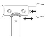
**1** Insert and secure the left and right handlebars by pressing the spring-loaded buttons and inserting them into the T-tube.
