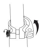
**Note:** The tension of the quick-release lever can be adjusted by tightening or loosening the Allen bolt. Be careful not to over-tighten. You should always be able to open and close the quick-release lever by hand and the T-tube should slide freely with the quick-release open.
