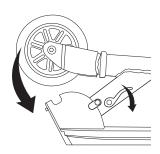
**3** To release the folding mechanism, put one foot on the deck plate and push joint release lever down. Raise handlebars up until securely locked in the upright position.
