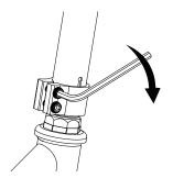
**2** With the front wheel pointed straight ahead, the handlebars square to the front wheel and the Razor Logo facing the front, tighten the clamp as shown. Tighten securely.
