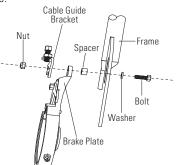
**9** Install the cable guide bracket to the frame and brake plate using bolt, washers, and nut. Do not tighten.
