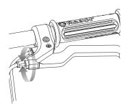
**1** To adjust the brake cable tension, thread the brake lever adjuster in or out 1/4 to 1/2 turn until the desired brake adjustment is attained. Most adjustments are complete at this step. If brake still needs further adjustment, proceed to step 2.
