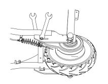
6 With two (2) 8 mm wrenches, remove the cable guide bracket from the frame and brake plate. Keep the bolt, washer, spacer, and nuts together.
