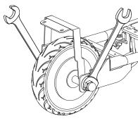
**7** With two (2) 19 mm wrenches, loosen the axle locknuts. Push down and remove the wheel from the frame.
