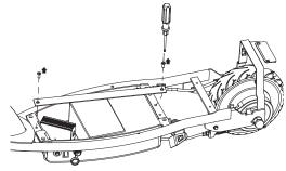
**2** Using a Phillips screwdriver remove the battery strap.
