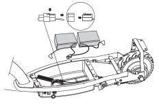
**3** Disconnect the battery wire connector from the control module and carefully remove the battery.
