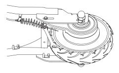
**5** With a 10 mm wrench, loosen the brake cable anchor bolt and disconnect the cable.
