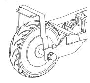
8 Install the new wheel on the frame. Put the wire into the guider. Hand tighten the rear axle locknuts.
