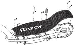
12 To install the replacement battery / hub motor, reverse steps 1 through 5. A: Small screw size, B: Allen bolt, C: Large screw size
