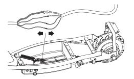
**4** Disconnect the motor wire connector from the control module and remove the wire from guider.
