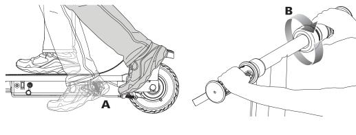
Note: Electric scooter must be moving at least 3 mph (5 km/h) while engaging throttle to engage motor.
