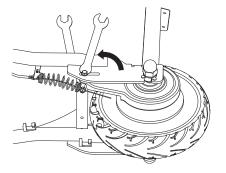
**11** Tighten the cable guide bracket bolt. Tighten the locknuts on the rear axle. Test the brake to verify proper function before riding. Readjust as needed.
