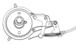
**10** Thread the brake cable through the brake adjuster barrel, through the large spring, and into the small hole in the side of the anchor bolt. Position the cable to the original location (as indicated by the slight cable kink) and tighten securely.
