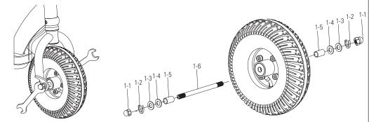
**1** Using two (2) 16 mm wrenches, loosen the axle bolts by turning the wrenches counter clockwise. Remove wheel and install replacement wheel. Note the sequence of the hardware.
