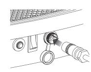
**2** Note: Make sure power switch is in the **OFF** position. Plug the charger into the charger port. The light on the charger should turn red during charging. The light will turn green again when charging is complete. **WARNING:** Use ONLY with the recommended charger. Batteries are only to be charged under adult supervision. The charger is not a toy. Always disconnect the charger before wiping down and/or cleaning the electric scooter with a damp cloth.
