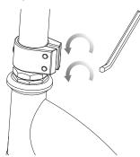
**1** Loosen the collar clamp. With a twisting motion, push and twist to slide the handlebar onto the fork.
