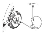
**1** Using a bicycle style tire pump equipped for a Schrader-type valve, inflate the front tire to the PSI indicated on the sidewall of the tire.
