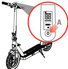
1 The cruise control mode is controlled by the power button on the display (A).
