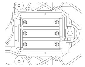
**Note:** When installing the batteries, please pay attention to the batteries' positive and negative side which must align with the positive and negative markings in the battery housing.
