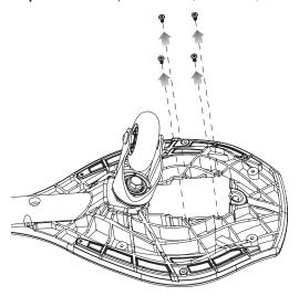
**1** Using a Phillips screwdriver, remove the four (4) screws from the battery cover.
