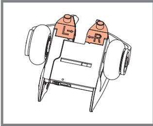
EN Installing/Replacing the Spark Pads/Skid Pads.
