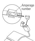
**2** Check all 3 fuses to see if the fuse(s) have burnt out. If the fuse(s) is(are) damaged, open the fuse cover. Remove any fuse that is damaged or burnt out and replace with a new one of equal amperage.
