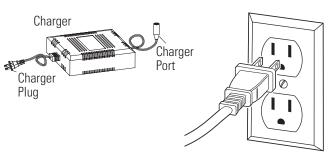
1 Plug the charger plug into a wall outlet. If the lights on the charger do not light up, check the power to the outlet. If necessary, try a different outlet.
