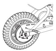
1 Loosen screw and remove chain guard.
