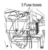
**1** Remove the seat fairing to locate the 3 fuse boxes attached to the batteries.
