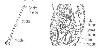
**1** Verify the spoke tension by shaking each spoke with your fingers. Spoke should not be loose from hub. Look for any play between where the spoke flanges attach to the hub. Try to turn the nipple using your fingers. You should not be able to spin any nipple by hand. If one or more spokes is loose, all spokes must be checked and need to be tightened with a spoke wrench.
