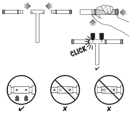
warning: Failure to properly engage the spring-loaded buttons may cause the handlebars to dislodge while riding and may cause you to lose control and fall. When correctly engaged, the handlebars will not rotate nor will they move sideways. Note that when properly engaged, the spring-loaded buttons are clearly visible in the holes on the T-bar.
