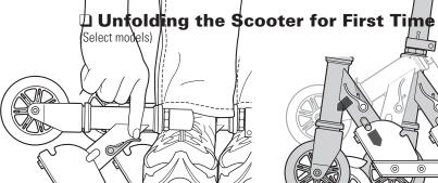
**1** To release the folding mechanism, place the scooter on the ground, put one foot on the deck plate and push joint release lever down. Raise T-bar up until it is securely locked in the upright position.
