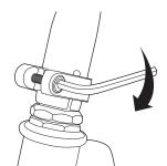
Using a 5 mm Allen wrench, check that the collar clamp bolt(s) are tightened securely. This item is tightened and quality inspected at the factory, but there is a slight chance that the effects of shipping or handling may have caused the bolt(s) to loosen.
