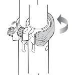
Note: The tension of the quick-release lever can be adjusted by manually tightening or loosening the Allen bolt. Be careful not to over-tighten. You should always be able to open and close the quick-release lever by hand and the T-bar should slide freely when the quick-release is open.
