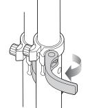
1 To adjust the height of the handlebars, open the quick-release lever and slide the T-bar to the desired position and resecure the quick release lever to lock into place. When the T-bar is raised to the maximum height, depress the push button located directly below the quick release lever to unlock the T-bar.
