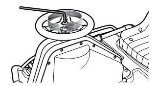
2 Using a 6 mm Allen wrench, tighten the steering bolt to secure the steering wheel in place.
