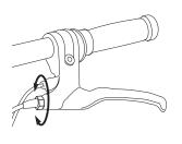
**1** To adjust the brake cable wire, thread the brake lever adjuster in or out 1/4 to 1/2 turn until the desired cable tension is attained.
