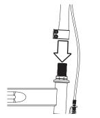
**1** Place the handlebar stem on the front fork.
