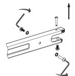
**1** Using two (2) 5 mm Allen wrenches, remove the two coupling bolts from the frame.
