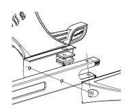
**2** Position the right and left foot platforms up to the frame and align holes.
