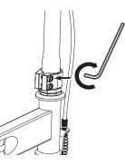
**2** Using a 5 mm Allen wrench to tighten the two (2) bolts on the collar clamp. The collar clamp is properly tightened when the handlebars cannot be twisted out of alignment with the front wheel. Make sure the handlebars are in line with the front wheel before tightening the bolts all the way.
