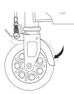
**2** Squeeze the brake lever to test the brake to make sure it is working properly. The front fender should clamp down and rub against the front wheel. If brake is not working properly, proceed to the next step.
