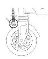
**3** If the brake is too tight or too loose, use a 8 mm wrench and a 3 mm Allen wrench to make adjustments as needed.
