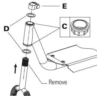
**4** Insert plastic headset ((C) - See 8, page 4) into the neck of the frame. Remove the protective black plastic cap from the top of the fork and slide one plastic washer (D) onto the fork before inserting the fork through the frame. Insert second plastic washer (D) onto the top of the fork and slide the collar clamp (E) on top of washer.
