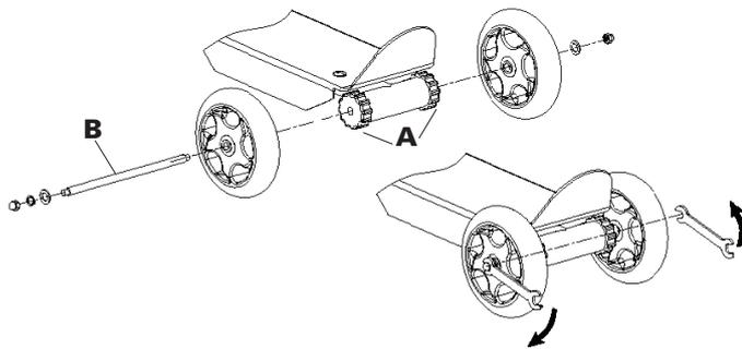
**3** Insert the rear tube covers ((A) - See 13-1, page 4). Slide rear axle bolt (B) through the frame and attach wheels to the end of the axle bolt. Insert washer and lock nut and tighten securely using a 13mm wrench.
