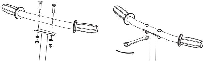
**1** Align the holes on the handlebars and the stem. Insert handlebar bolts into the top of the handlebar and through the stem. Install the washers and nuts onto the bottom of the handlebar bolts. Tighten securely into place using a 10mm wrench.
