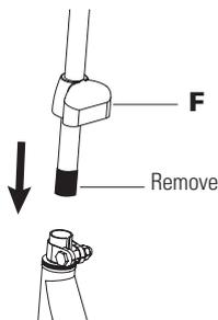
**5** Remove the protective black plastic cap from bottom of stem and slide collar clamp cover (F) up to the middle of the stem. Insert the stem into the fork.
