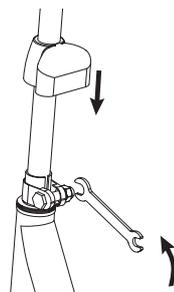
**6** Using a 13 mm wrench, tighten the bolt on the collar clamp until the handlebars are locked securely into place. Slide the collar clamp cover down over the collar clamp.
