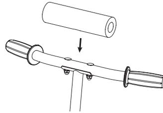
**2** Place the handlebar pad over the handlebars and secure tightly with the velcro cover.
