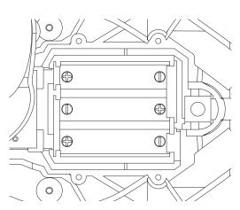
**Note:** When installing the batteries, please pay attention to the batteries' positive and negative side which must align with the positive and negative markings in the battery housing.
