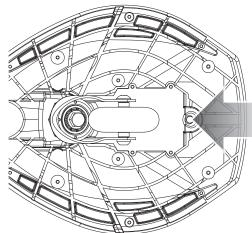
**4** Insert the new AA batteries and replace the cover and four (4) screws using a Phillips screwdriver.
