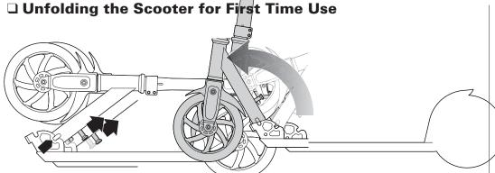
**1** To release the folding mechanism, place the scooter on the ground, put one foot on the deck plate and pull the joint release lever up. Raise T-bar up until it is securely locked in the upright position.
