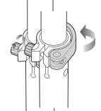
Note: The tension of the quick-release lever can be adjusted by manually tightening or loosening the Allen bolt. Be careful not to over-tighten. You should always be able to open and close the quick-release lever by hand and the T-bar should slide freely when the quick-release is open.
