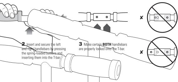
warning: Failure to properly engage the spring-loaded buttons may cause the handlebars to dislodge while riding and may cause you to lose control and fall. When correctly engaged the handlebars will not rotate nor will they move sideways. Note that when properly engaged, the spring-loaded buttons are clearly visible in the holes on the T-bar.
