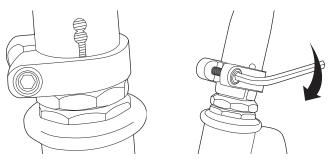
Using a 5 mm Allen wrench, check that the collar clamp bolt(s) are tightened securely. This item is tightened and quality inspected at the factory, but there is a slight chance that the effects of shipping or handling may have caused the bolt(s) to loosen.
