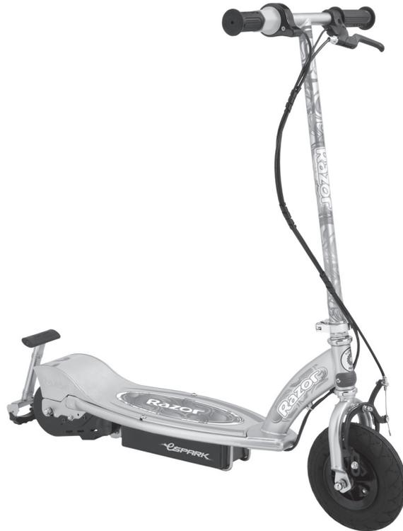
**⚠ NOTE:** The eSpark must be traveling up to 3mph before motor will engage. Kick start up to 3mph while twisting the throttle to engage motor.
