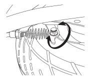
**2** If the brake is too tight or too loose, use a 10mm open wrench to loosen the nut for additional adjustment on the brake cable. Securely tighten the nut when finished.
