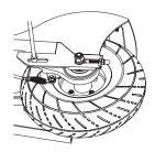
**3** With two 8mm wrenches, loosen brake housing anchor and disconnect. Keep the spacer and bolts together.
