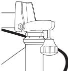
**3** Slide the guill into the fork until it bottoms on the headset
