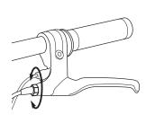
**1** To adjust the brake cable play, thread the brake lever adjuster in or out 1/4 to 1/2 turn until the desired brake adjustment is attained. Most adjustments are complete at this step. If brake still needs further adjustment, proceed to step 2.
