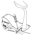
**3** Place the seat post on the deck and secure using the same 4 screws.
