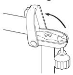
1 Loosen the locking knob and swing to the 6 o'clock position to unfold the handlebar.
