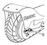
**1** With a Phillips screwdriver, loosen the two screws and remove the chain guard.
