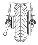
**3** Using a 10mm wrench, tighten the tension adjusters on the axle 1/8 to 1/4 turn to fine-tune the chain tension. Both adjusters must be tightened the exact same amount to maintain wheel alignment.
