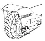
**2** Open the round cover located on the chain cover by sliding the cover upward. Align the opening in the drive sprocket with the valve stem. Thread the adapter completely onto the valve stem and attach the pump. Inflate to the PSI indicated on the tire sidewall.
