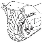
**4** Once the tension is correct, tighten the axle bolts and brake housing anchor bolt. Test ride the scooter. Readjust as needed.
