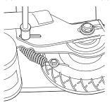
**2** Using two 8mm wrenches, loosen the brake housing anchor bolt which is located in the long slot on the left side of the rear fork.
