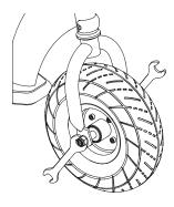
1 Using two 17mm wrenches, loosen the front axle bolts by turning the wrenches counter clockwise.
