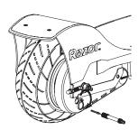
**3** Remove valve extender immediately after inflating and close the round cover.
