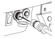
**1** Turn **OFF** power switch before charging. Plug the charger into the charger port on the electric scooter.
