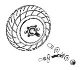
**6** Remove wheel. Note the sequence of the hardware.
