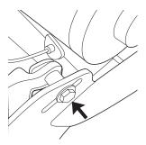
**8** To hook up the brake housing anchor, align the cable guide adjuster and install the spacer and bolt. Do not tighten until final step.
