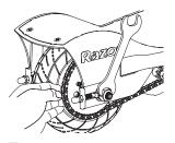
**7** Install new chain or wheel by maneuvering the chain onto the sprocket and slipping the axle into the slots on the frame.
