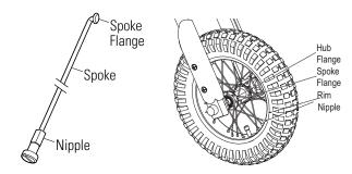
**1** Verify the spoke tension by grasping and shaking each spoke. Spoke should not be loose from hub. Look for any play between the spoke flanges where it mates with the hub. Try to turn the nipple using your fingers. You should not be able to spin any nipple by hand. If one or more spokes is loose, all spokes should be checked and tightened with a spoke wrench if needed.
