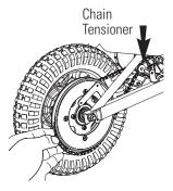
**5** Install the new chain or wheel by slipping the chain around the axle. Slide the axle into the slots on the frame. Slide the chain tensioner down and maneuver the chain onto the sprocket on the rear wheel and motor.
