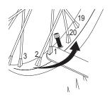
**2** Start with spoke closest to the tire valve stem and tighten each nipple, in sequence, exactly 1/4 to 1/2 turn. A single 1/4 to 1/2 turn may not be enough to bring the spokes into proper tension. Continue tightening all spokes no more than 1/2 turn in sequence until all spokes are tight.
