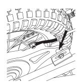
**6** To re-attach the brake housing anchor, align the cable guide adjuster and install the spacer and bolt. Do not tighten until final step.
