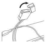
**2** Locate the fuse box attached to the batteries. Open the fuse cover to expose the fuse.
