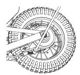
**2** With a 10mm wrench, loosen the brake cable anchor and disconnect the cable.
