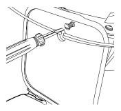
**1** Remove screw from front fork. Align the number plate with the hole in the fork and tighten with a Philips screw driver.
