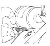
**7** Install the brake spring and thread the cable wire into the cable anchor. Thread the cable to its original position and tighten securely.
