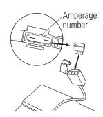
**3** Remove the fuse and replace with a new one of equal amperage. Requires 30 amp fuse. Close the fuse cover and reattach the batery cover.
