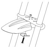
**1** Align fender with the hole in the fork and insert the bolt. Tighten securely using a 10mm Wrench and 5mm Allen Wrench.
