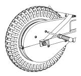
**1** Loosen screws and remove chain guard.
