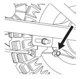
**2** If the brake has too much slack, use a 10mm open wrench to loosen the brake anchor cable for additional adjustment.
