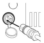
**1** Turn power **OFF** before charging. Plug the charger into the charger port on the motor bike.
