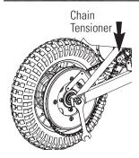
4 With two 15mm wrenches, loosen the axle. Push the chain tensioner down to loosen the chain and pull the wheel out.
