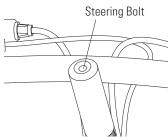
**5** Securely tighten bolt using 6 mm Allen wrench.
