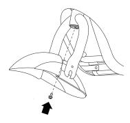
**2** Insert the front fender into the front fork and tighten the screw using a Phillips screwdriver.
