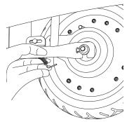
**7** Thread the brake cable through the brake adjuster barrel, through the large spring, and into the small hole in the side of the anchor bolt. Position the cable to the original location (as indicated by the slight cable kink) and tighten securely.
