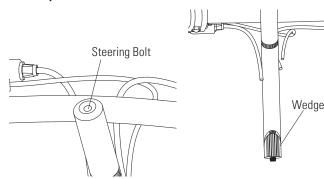
1 Using a 6 mm Allen wrench, loosen steering bolt in four (4) complete turns so that the wedge is loose and not touching steering tube.
