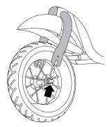
2 Insert the new wheel into the front fork with the lock washers on the outside of the fork. See step #3.
