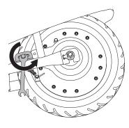
**4** Using two (2) 8 mm wrenches, loosen and remove the bolt and lock nut from the cable guide bracket.
