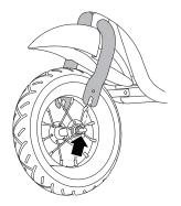
**3** Insert the wheel into the front fork with the lock washers on the outside of the fork.
