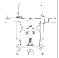
2 Facing the front of the Pocket Mod Petite, position the handlebars so the throttle is on your right and the brake lever is on your left (the red "SAFE ZONE" print will be facing you). Align wedge inside handlebar tube. Note: Plastic cover needs to be removed prior to installing the handlebars.
