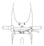
**3b** The throttle should now be on your left and the brake lever on your right.
