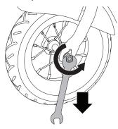
1 Remove the nuts on both sides of the front axle using a 14 mm wrench then remove the lock washers and remove the wheel from the fork.
