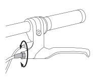
**1** To adjust the tension, thread the brake lever adjuster on the hand brake in or out 1/4 to 1/2 turn until the desired brake adjustment is attained. Most adjustments are complete at this step. If brake still needs further adjustment, proceed to step 2.
