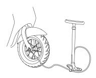
Using a bicycle tire pump equipped for a Schrader valve, inflate the tires to the PSI indicated on the sidewall of the tires.
