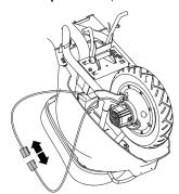
**1** Locate and disconnect motor from controller.
