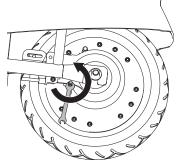
**2** If brake is too tight or has too much slack, use a 10 mm wrench to loosen the nut for additional adjustment on the brake cable on the rear wheel. Securely tighten nut when done.
