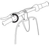
**1** Adjust angle of the brake lever to a comfortable position for the rider by turning back and forth.
