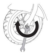
**5** Tighten the nuts using two (2) 14 mm wrenches.
