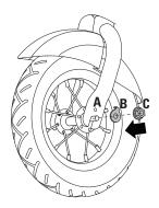
3 Insert tab on the lock washer (B) into the hole (A) on the front fork and then place the nuts (C) on top of the lock washer (B).
