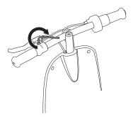
**2** Securely tighten the bolt using a 5 mm Allen wrench.
