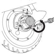
**2** Using a Phillips screwdriver, loosen and remove three (3) screws from motor cover.
