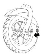
**4** Insert the tab on the lock washer into the hole on the front fork.
