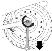
**5** With 17 mm wrench, loosen the nut. Remove wheel/hub motor.
