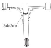
4 Slowly slide the handlebars up to make certain that the bar is in the "SAFE ZONE". Failure to secure the handlebars within the "SAFE ZONE" can cause the handlebars to come out while riding.
