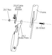
6 Install the cable guide bracket to the frame and brake plate using bolt, washers, and nut. Do not tighten.
