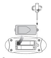
**3** Re-attach battery cover and securely tighten in place with screw.
