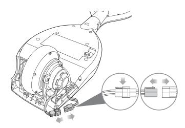
**2** Disconnect the motor connector from the control module.
