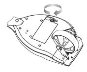
**4** Re-attach battery cover and securely tighten in place with screw.
