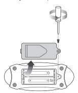
**1** Loosen Phillips screw on battery cover and remove cover. Remove old batteries and properly dispose.
