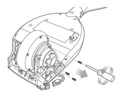
**4** Loosen the three (3) Phillips screws that attach the motor housing to the frame. Remove rear wheel.
