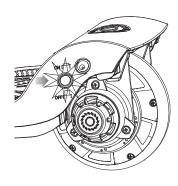
**6** If the light on the product continues to flash quickly, turn power switch on the remote to the **OFF** position and repeat steps 3-4 until remote is paired.
