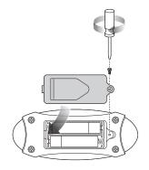
**3** Re-attach battery cover and securely tighten in place with screw.
