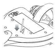
**3** Using a small object, **gently** tap the center of the pairing button. The light on the power button should now be flashing quickly.
