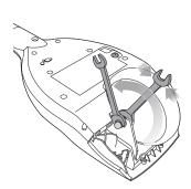
**3** Using a 13 mm wrench, loosen the outside locknut (11-6). Use a 13 mm wrench to prevent the inside nut (11-3) from turning.
