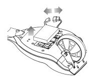
**2** Disconnect the battery connector from the control module and carefully remove the battery from product.
