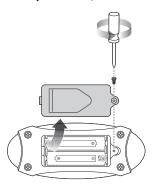
**1** Loosen Phillip screw on battery cover and remove cover.
