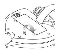
**2** Turn product over. Open the pairing button cover located underneath the rear platform.
