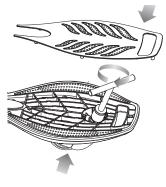
**3** Insert replacement caster. Secure in place with nut removed in step 2.
