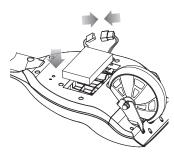
**3** Install replacement battery. Re-connect the battery connector to the control module.
