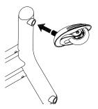
**1** Locate the threaded hole on the rear underside of the frame. Screw caster wheel into hole.
