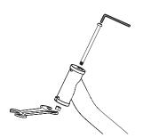
**1** Remove the steering bolt and locknut from the frame assembly with a 13mm open wrench and 5mm allen wrench.
