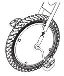
**2** Insert the wheel assembly into the front fork assembly and align holes.
