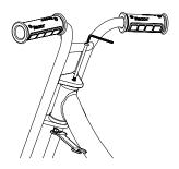
**4** Re-insert the steering bolt and secure with locknut using a 13mm open wrench and 5mm allen wrench.
