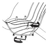
**3** Tighten bolts using two 5mm allen wrenches. One on top and one on bottom.
