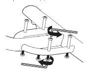
**1** Remove the four coupling bolts from the frame using two 5mm allen wrenches. One on top and one on bottom.
