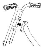
**2** Insert the front fork into the frame assembly.
