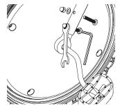
**3** Re-insert the coupling bolts through the front fork and secure with allen wrench and open wrench.
