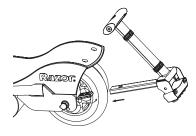
**1** Using two (2) 5mm Allen wrenches remove the coupling bolt that is attached to the end of the metal bar of the Spark bar. Slide the Spark bar onto the metal bar located on the opposte side of the chain. Push down on the Spark bar and slide the bar all the way on until the holes are aligned.
