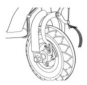
**1** Using a 10mm open wrench, loosen the brake cable bolt.
