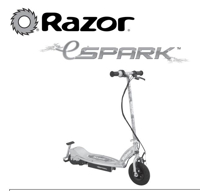
**NOTE:** The eSpark must be traveling up to 3mph before motor will engage. Kick start up to 3mph while twisting the throttle to engage motor.
