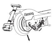
**3** To loosen the chain, push the tensioner down to create some slack in the chain.
