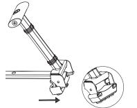
**1** Using your thumbs, press tabs (A & B) on both sides of the cartridge to release from the bracket. Slide cartridge away from you and in place.
