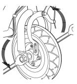
**2** Using two 17mm open wrenches, loosen the locknuts by turning the wrenches counter clockwise. Remove wheel and install replacement wheel.
