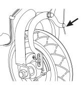
**2** If brake is too tight or has too much slack, use a 10mm open wrench to loosen the brake cable and adjust accordingly.
