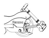
**2** Re-insert the coupling bolt through the metal bar and tighten until Spark bar is locked securely in place.
