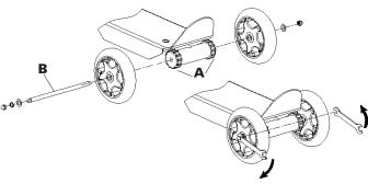
**3** Insert the rear tube covers ((A) - See 13-1, page 4). Slide rear axle bolt (B) through the frame and attach wheels to the end of the axle bolt. Insert washer and lock nut and tighten securely using a 13mm wrench.
