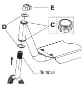
4 Insert plastic headset ((C) - See 8, page 4) into the neck of the frame. Remove the protective black plastic cap from the top of the fork and slide one plastic washer (D) onto the fork <a href="mailto:before">before</a> inserting the fork through the frame. Insert second plastic washer (D) onto the top of the fork and slide the collar clamp (E) on top of washer.
