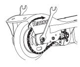
**6** With two 13mm wrenches, re-tighten the locknuts.
