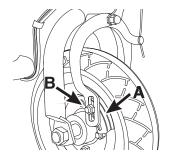
**3** Inspect the brake pads (A) for proper alignment against the wheel or excess wear. To realign brake pads, loosen the fixing nut (B) and adjust the pad to contact the rim. Retighten and test. Readjust as needed.
