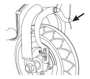
**2** If brake is too tight or has too much slack, use a 10mm open wrench to loosen the brake cable and adjust accordingly.
