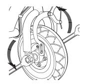
**2** Using two 17mm wrenches, loosen the locknuts by turning the wrenches counter clockwise. Remove wheel and install replacement wheel.
