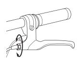
**1** To adjust the brake cable play, thread the brake lever adjuster in or out 1/4 to 1/2 turn until the desired brake adjustment is attained. Most adjustments are complete at this step. If brake still needs further adjustment, proceed to step 2.
