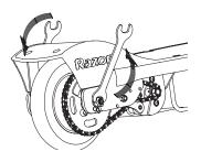
**2** Using two 13mm wrenches, loosen the locknuts by turning the wrenches counter clockwise.
