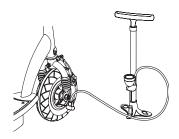
1 Using a bicycle style tire pump equipped for a Schradertype valve, inflate the front tire to the correct PSI indicated on the sidewall of the tire.
