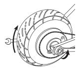
With two 17mm wrenches, loosen the axle. Push the wheel forward to loosen the chain and remove from rear and front sprocket.
