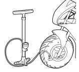
**1** Using a bicycle-style tire pump equipped for a Schrader-type valve, inflate the front tire to the PSI indicated on the sidewall of the tire.
