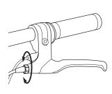
1 To adjust the play, thread the brake lever adjuster in or out 1/4 to 1/2 turn until the desired brake adjustment is attained. Most adjustments are complete at this step. If brake still needs further adjustment, proceed to step 2.
