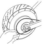
Install the new chain or wheel by slipping the chain around the axle. Slide the axle into the slots on the frame. Maneuver the chain onto the rear sprocket and front sprocket.
