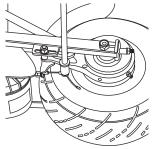
With a 10mm wrench, loosen the brake cable anchor and disconnect the cable.
