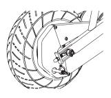
2 Push open the access cover and align the access hole in the drive sprocket with the tire valve. Thread the adapter completely onto the valve and attache the pump and inflate to the PSI indicated on the tire sidewall. Push the access hole cover back.
