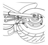
**3** With two 8mm wrenches, loosen brake housing anchor and disconnect. Keep the spacer and washers together.
