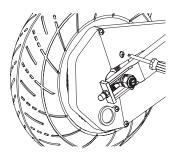
1 Loosen screws and remove chain guard.
