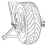
Loosen and remove both axle adjuster nuts.
