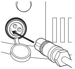
**1** Plug the charger port into the port on the electric motor bike. The charger works with the power switch in either the on or off position.
