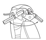
**1** Swing the handlebars outward as shown. You may have to loosen the clamps to allow the bar to pivot on the fork.
