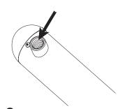
**3** If you're having trouble threading the caster into frame, use a rag or small brush with a little WD-40® to remove any excess particles that may be caught in or around the threading within the frame.
