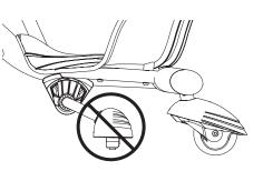
NEVER push down directly on the Spark Bar, spark cartridge or spark cartridge cover itself.
