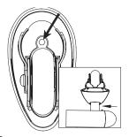
**2** Using a 5mm Allen wrench, tighten the hex bolt located on the underside of the wheel cover until the caster bolt is all the way inside the frame.
