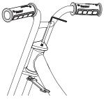
**4** Re-insert the steering bolt and secure with locknut using a wrench.
