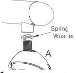
**1** Insert the caster bolt into the frame. If aligned correctly, the caster thread should go half way into the frame with no resistance.
