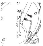
**3** Re-insert the coupling bolts through the front fork and tighten securely.
