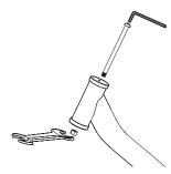
1 Remove the steering bolt and locknut from the frame assembly with a 13mm open wrench and 5mm Allen wrench.
