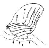
**2** Align the four holes in seat with the four holes in frame. Insert coupling bolts through the top and bottom of the frame.
