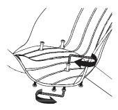
**3** Tighten bolts using two 5mm Allen wrenches; one on top and one on bottom.
