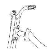
2 Insert the front fork into the frame assembly.
