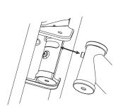
**3** Be sure to properly align slot in headset tube with pin on fork as shown.
