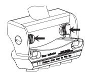
**1** Using your thumbs, press tabs on both sides of the cartridge to release from the bracket. Slide cartridge away from you and remove from bracket.
