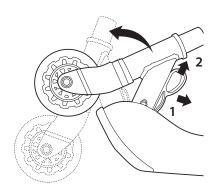
**1** Pull the folding release lever away and up to raise the front fork into the upright position.
