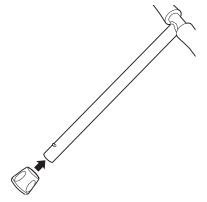
**3** Slide the steering clamp cover onto the T-bar.
