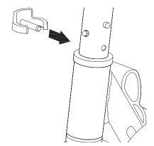
**5** Insert the "E" shaped fixed pin into the open hole on the front fork assembly to secure T-bar.
