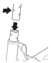
**4** Insert the T-bar into the front fork assembly using your thumb to depress the button on the T-Bar until it "locks" into place.
