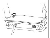
**3** Close the fuse box and reattach the deck plate by reversing instructions in Step# 1.
