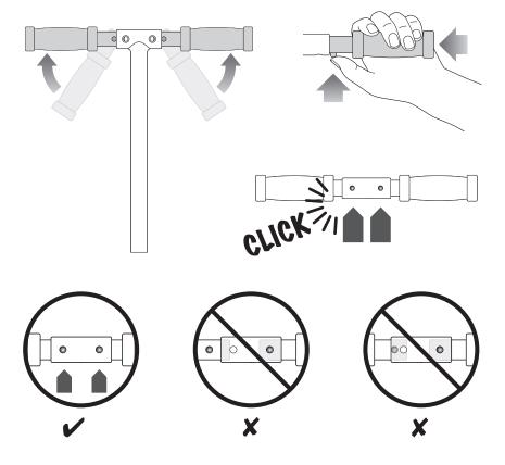
warning: Failure to properly engage the spring-loaded buttons may cause the handlebars to dislodge while riding and may cause you to lose control and fall. When correctly engaged, the handlebars will not rotate nor will they move sideways, and the spring-loaded buttons will be clearly visible in the holes on the T-Bar.
