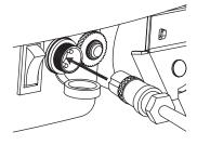
**1** Turn **OFF** power switch before charging. Plug the charger into the charger port on the electric scooter.
