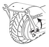
**1** Using two 17mm wrenches, loosen the rear axle bolts by turning the wrenches counter clockwise.
