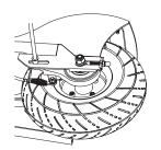
**3** With two 8mm wrenches, loosen brake housing anchor and disconnect. Keep the spacer and bolts together.
