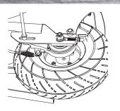
**12** Tighten the brake housing anchor securely. Test ride. Readjust as needed.
