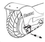
**3** Remove valve extender immediately after inflating and close the round cover.
