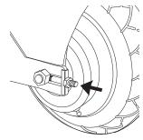
**10** Install the axle adjusters and axle nuts. Tighten until they just barely hold the hardware in place.
