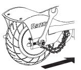
**5** With two 17mm wrenches, loosen the axle. Slide the wheel forward to loosen the chain.
