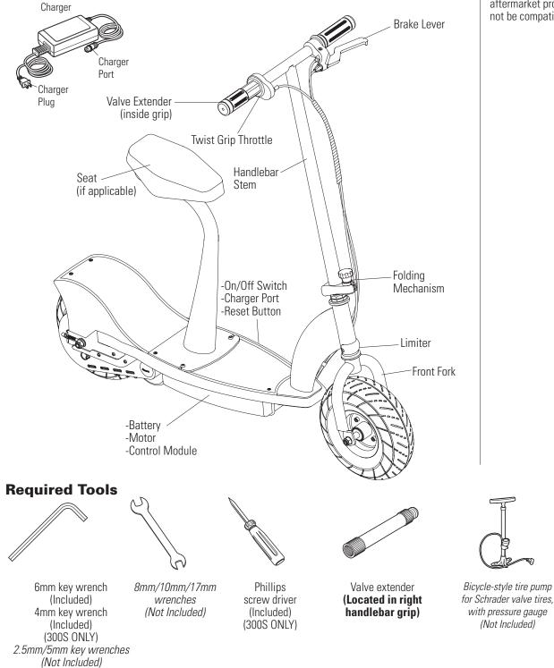
A warning: DO NOT USE NON-RAZOR PRODUCTS WITH YOUR RAZOR ELECTRIC SCOOTER. The scooter has been built to certain Razor design specifications. The original equipment supplied at the time of sale was selected on the basis of its compatibility with the frame, fork and all other parts. Certain aftermarket products may or may not be compatible.
