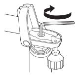
**4** Using a 6mm hexagonal key wrench, tighten the wedge by turning the bolt clockwise. The wedge is properly tightened when the handlebars cannot be twisted out of alignment with the front wheel.
