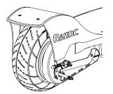
**2** Open the round cover located on the chain cover by sliding the cover upward. Align the opening in the drive sprocket with the valve stem. Thread the adapter completely onto the valve stem and attach the pump. Inflate to the PSI indicated on the tire sidewall.
