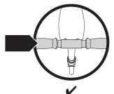
warning: Failure to properly engage the spring-loaded buttons may cause the handlebars to dislodge while riding and may cause rider to lose control and fall. When correctly engaged, the handlebars will not rotate nor move sideways, and the spring-loaded buttons will be clearly visible in the holes on the T-bar.
