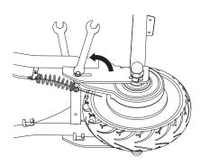
**11** Tighten the cable guide bracket bolt. Tighten the locknuts on the rear axle. Test the brake to verify proper function before riding. Readjust as needed.
