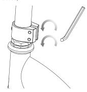
**2** With the front wheel pointed straight ahead and the handlebars square to the front wheel, tighten both bolts on the clamp as shown with a 5 mm Allen wrench. Tighten securely.
