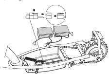
3 Disconnect the battery wire connector from the control module and carefully remove the battery.
