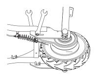
6 With two (2) 8 mm wrenches, remove the cable guide bracket from the frame and brake plate. Keep the bolt, washer, spacer, and nuts together.
