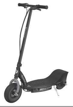
**NOTE:** The unit must be traveling at least 3 mph (5 km/h) before motor will engage. Kick start to at least 3 mph (5 km/h) while applying throttle to engage motor.
