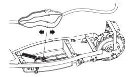
**4** Disconnect the motor wire connector from the control module and remove the wire from guider.
