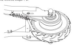
**5** With a 10 mm wrench, loosen the brake cable anchor bolt and disconnect the cable.
