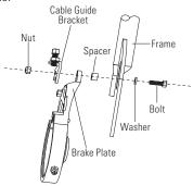
**9** Install the cable guide bracket to the frame and brake plate using bolt, washers, and nut. Do not tighten.
