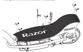
1 Using a Phillips screwdriver and 4 mm Allen wrench remove the six (6) screws and two (2) Allen bolts and remove the deck plate. A: Small screw size, B: Allen bolt, C: Large screw size
