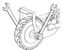
**7** With two (2) 19 mm wrenches, loosen the axle locknuts. Push down and remove the wheel from the frame.
