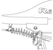
**2** If the brake is too tight or too loose, use a 10 mm wrench to loosen the nut for additional adjustment on the brake cable. Securely tighten the nut when finished.
