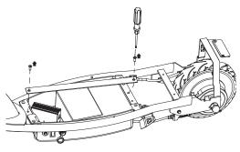
**2** Using a Phillips screwdriver remove the battery strap.
