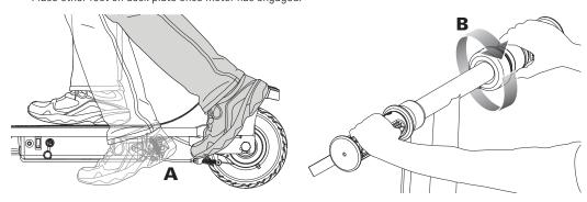
Note: Electric scooter must be moving at least 3 mph (5 km/h) while engaging throttle to engage motor.
