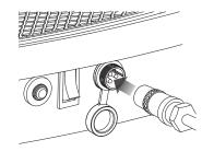
**2 Note:** Make sure power switch is in the **OFF** position. Plug the charger into the charger port. The light on the charger should turn red during charging. The light will turn green again when charging is complete.
