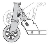
**Note:** The joint release lever is spring-loaded and will automatically lock in the upright position when fully upright.
