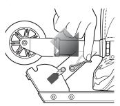
1 To release the folding mechanism, place the scooter on the ground, put one foot on the deck plate and push joint release lever down. Raise T-bar up until it is securely locked in the upright position.
