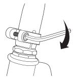
Using a 5 mm Allen wrench, check that the collar clamp bolt(s) are tightened securely. This item is tightened and quality inspected at the factory, but there is a slight chance that the effects of shipping or handling may have caused the bolt(s) to loosen.
