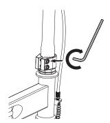
**2** Using a 5 mm Allen wrench to tighten the two (2) bolts on the collar clamp. The collar clamp is properly tightened when the handlebars cannot be twisted out of alignment with the front wheel. Make sure the handlebars are in line with the front wheel before tightening the bolts all the way.
