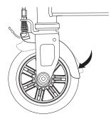
**2** Squeeze the brake lever to test the brake to make sure it is working properly. The front fender should clamp down and rub against the front wheel. If brake is not working properly, proceed to the next step.
