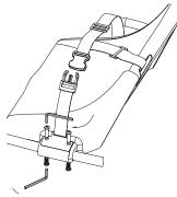
**1** Position the seat over the frame and align it with the holes in the frame. Align the safety belt anchor holes to the holes in the seat and frame with the lap/shoulder assembly on the left and the receiver latch on the right. Insert the screws and tighten securely.
