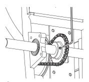
**3** Use a 3mm wrench to loosen the sprocket.
