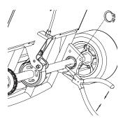
**4** Remove c-clips on the axle between the two bearings.
