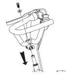
**2** Untangle the wires. Insert the steering wheel, washer and screw into the steering column as shown.
