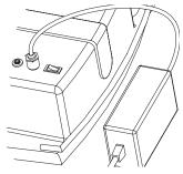
**1** Plug the charger into the port on the Ground Force Drifter. Make sure the power switch is in the "OFF" position.
