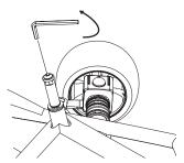
**1** Using a 5mm Allen wrench, loosen the screw located in the steering column.
