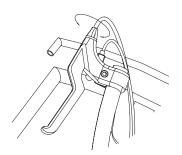
**1** To adjust the brake, thread the adjuster in or out 1/4 to 1/2 turns until the desired brake adjustment is attained.
