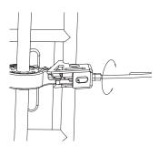
2 If the adjuster is threaded outward and the brake still has too much slack, use the auxiliary adjuster at the rear brake for additional adjustments.
