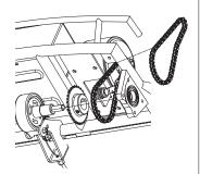
**6** When the axle end is clear of the bearing hanger, remove and replace the chain. Reverse this procedure to reassemble.
