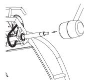
**5** Lightly tap the end of the axle with a rubber mallet. DO NOT USE A HAMMER as this will damage the thread. The brake drum and pulley must be slid along the axle as your tapping progresses.
