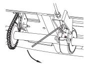
**2** Use a 3mm wrench to loosen the brake.
