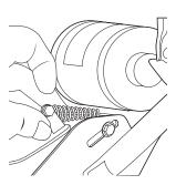
**9** Install the brake spring and thread the cable wire into the cable anchor. Thread the cable to its original position and tighten securely.
