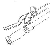
**1** To adjust brake cable play, thread the brake lever adjuster in or out 1/4 to 1/2 turn until the desired brake adjustment is attained. Most adjustments are complete at this step. If brake still needs further adjustment, proceed to step 2.
